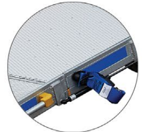
Gas spring between the two platforms
