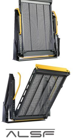
The automatic, twin-arm, electro-hydraulic lifts in the **BB** Series have a one-piece platform. Thanks to a two-button control unit and the use of top quality materials, these devices are not only user friendly, they are also extremely reliable. Available in a wide range of sizes, they can be internally rear or side mounted in a wide variety of people carriers.
